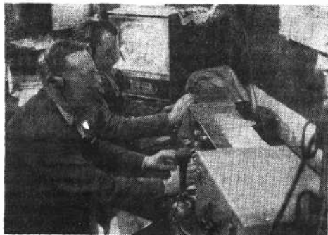
Right of stage: Master sound and vision mixers, with three pre-view monitors out of picture, and transmission monitor at rear. Monitor at rear L is in the studio.
